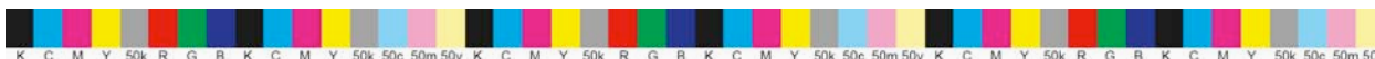
Basic press control bar color patches – layout may vary – (not suitable for G7 press control)
