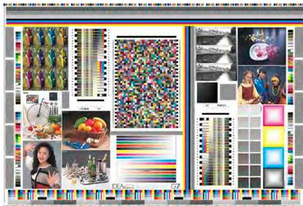
**FIGURE E.1** A typical 28" x 40" G7 press form
