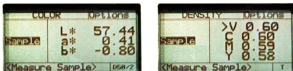
FIGURE E.12 Typical gray balance reading in Lab (left) and CMY density (right).
