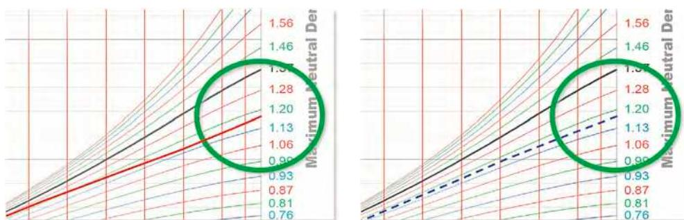
FIGURE 3.11 Left: The nearest two pre-printed graphs above and below the sample graph are 1.20 and 1.13. Right: Drawing a new target graph between the 1.13 and 1.20 graphs.
