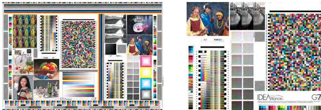
FIGURE 3.7 Typical G7 press form (left) and proofing form (right)
