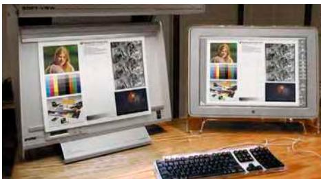
**FIGURE F.1** Typical soft proofing setup with a dimmable viewing booth matched to display brightness
